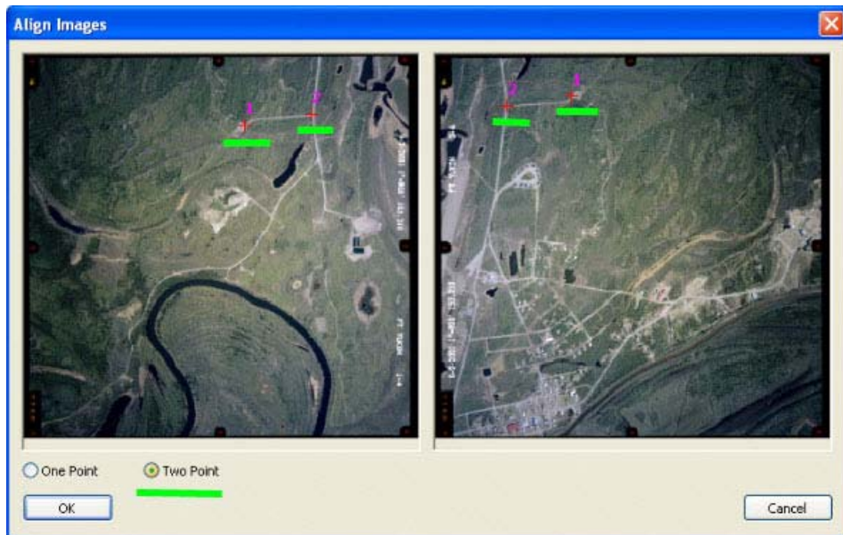
These images are approximately 180 degrees from each other. Use Two Point and digitize two similar ground features in the same order.
